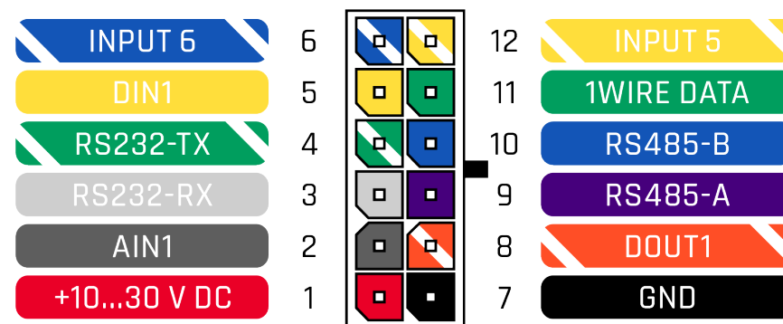
Figure 2 FMB125 2x6 socket pinout
